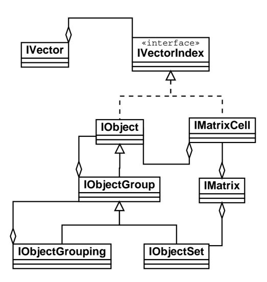
Figure 3.1: UML. Part of the Infomat data-structure
